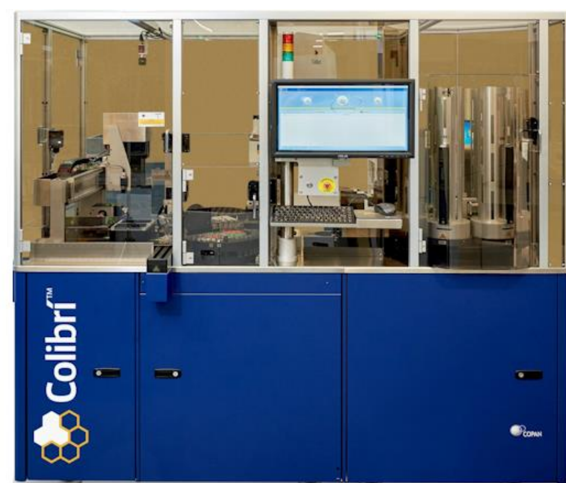
Figure 2. A picture of the Copan's Colibri® we used in this validation, a device designed to automatize colony picking, and preparation of targets for the identification of bacteria and yeasts through MALDI-TOF technology, and bacterial suspensions for AST. The Colibri® coupled with the Radian in-Line Carousel® and the Radian Expert System® for antibiotic disk dispensing and halo interpretation, provide a fully automated solution for antimicrobial disk diffusion susceptibility testing.
